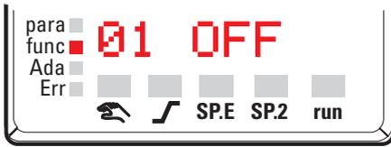
Programmer is in reset and the internal controller set-point is effective. Segment or program number and **OFF** are displayed (configurable with BlueControl: Configuration → Other → PDis3).
