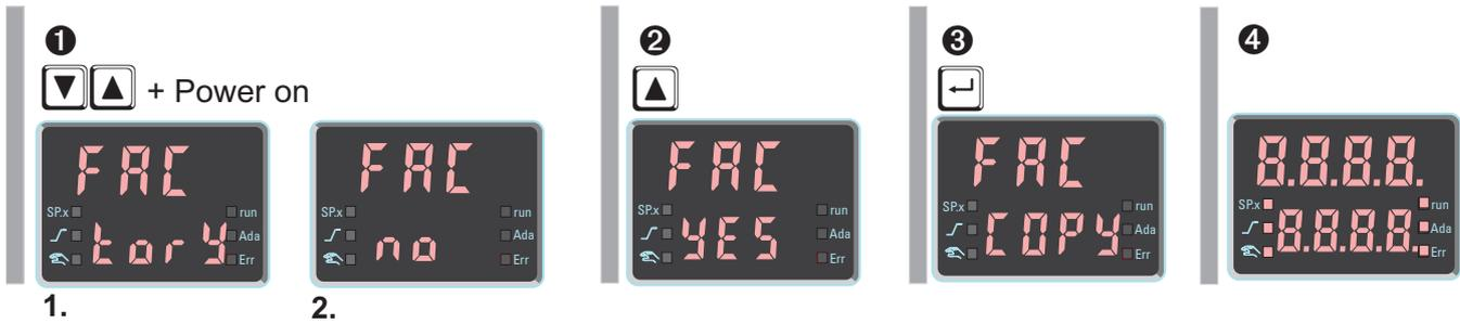
The operator must keep the keys increment and decrement pressed during power-on.
